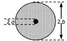
c) Hence derive an expression for the capacitance per unit length of the coaxial cable. (4 marks)
