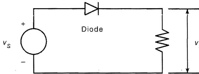
Figure 1: Ideal diode circuit
